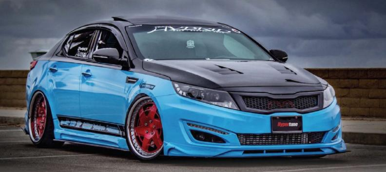
It all starts with the Aeroflow front bumper with Voltex extensions and a Morris Club front chin spoiler. Flowing into the Garcia Factory side skirts complimented by the Karbon Koncepts carbon fibre side skirt extensions, the lines of the car flow end at the Garcia Factory rear bumper extensions together with a Karbon Koncepts carbon fibre rear bumper diffuser.
