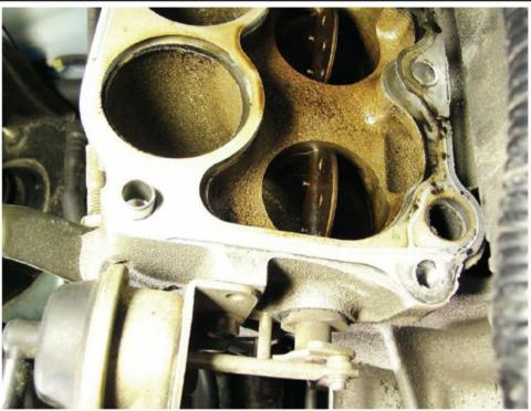
The image shows a shaft that controls a set of butterflys; the vacuum modulated (a bell-shaped modulator with a vacuum line attached to it) shaft's rotates and re-position the butterflys which in turn changes the manifold's properties. Current ones operates electronically.
